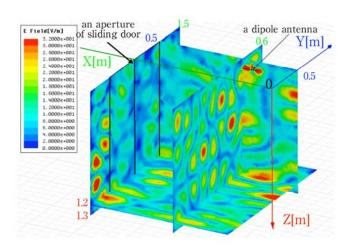
Figure 4 Snapshot of spatial distribution of intensity in elevator model, obtained using HFSS. Parameters are the same as those shown in Fig. 3. The door of the elevator, whose area is specified by X=1.5, Y:[-0.45, 0.45] and Z:[0, 1.3], is kept fully open. For details, see Appendix and ref. 19.
