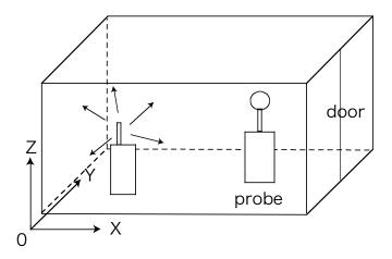
Figure 1 Installation of radiation source (FM transmitter) and probe.
