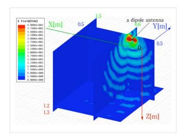
Figure 5 Snapshot of spatial distribution of intensity in the case without reflection. Parameters are the same as those for the elevator model, except for the boundary condition. For details, see Appendix and ref. 20.
