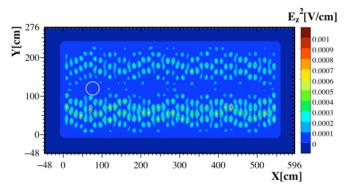
Figure 6 Snapshot of spatial distribution of intensity in 2D container model simulated by FDTD method. We set a radiation source and a human model as (X,Y)=(70,66) and (76,120), respectively. For details, see Appendix and ref. 22.
